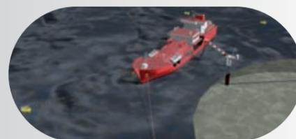
For locations with mild environmental conditions a conventional buoy mooring (CBM) terminal system can be designed for standard LNG carriers.
