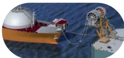
For the less benign and harsh environments a stern to bow transfer system has been designed. The qualification of this tandem LNG transfer system follows the RPA203 technology qualification process of DNV.
