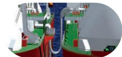
To allow flexible and efficient operation of offshore production facilities, it may be essential that for the transfer of LNG standard carriers can be utilized. This requires the transfer of LNG to take place at the mid-ship manifold.
