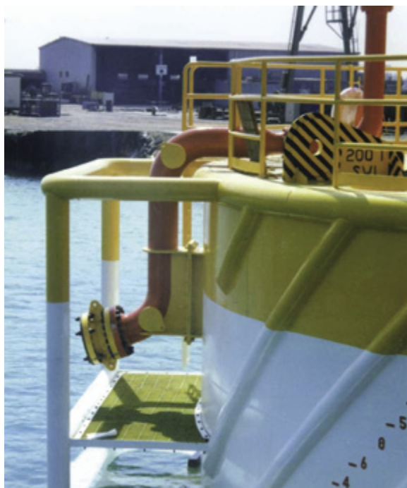
Woodside, Legendre Field Australia; Overboard piping solid connected to buoy and well protected
