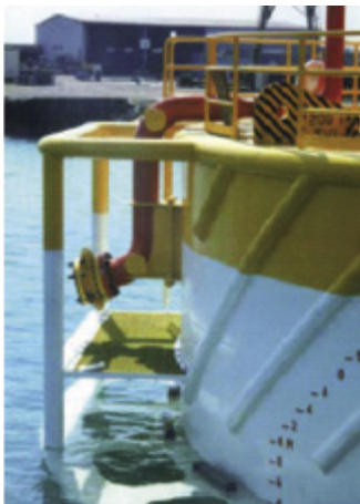
Overboard piping directly connected to buoy hull – strong support
