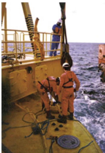
Personnel on the deck of a turntable buoy near to the rotating arm of the turntable which can move. The personnel is not protected by a handrailing.
