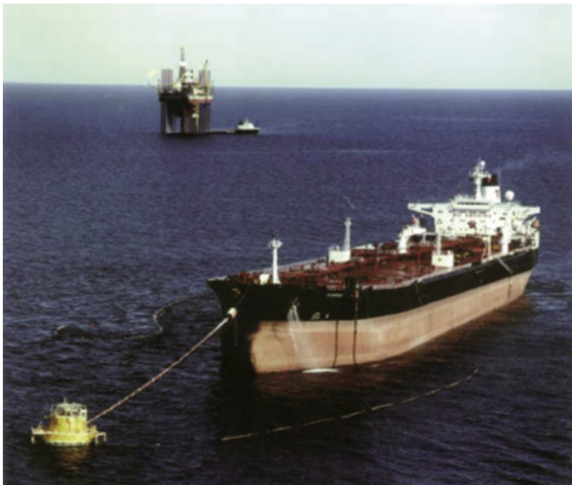
Apache, Stag Field, Australia, FSO moored to Turret Buoy
