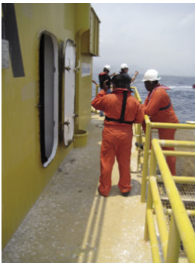
Personnel on deck of a Turret Buoy. Safety: no moving parts; safety handrail around the perimeter of the buoy. Also visible is the large boat landing
