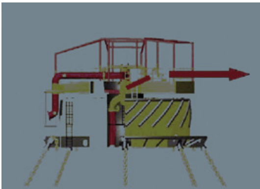
Turntable buoy: external loads on the turntable will pass 100% through the main bearing
