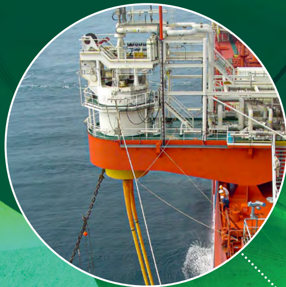
An external outrigger configuration with disconnectable buoy is also available
